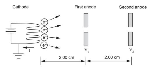
Assume the average initial velocity of a thermal electron is zero. The anode voltages are  $V_1 = 1500$  V and  $V_2 = 4500$  V and the distances between the cathode and anodes are as shown above.
