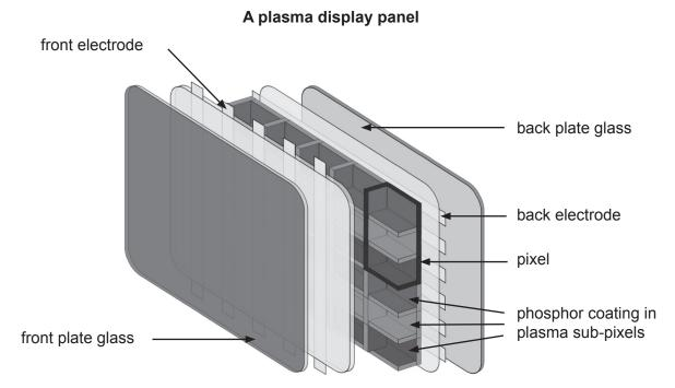
Control circuitry creates a voltage difference between the electrodes at the front and back of a sub-pixel. This sends a pulse of current through the sub-pixel. Some of the gas atoms in the sub-pixel become ionised, creating an electrically-conducting plasma consisting of atoms, free electrons and ions.
